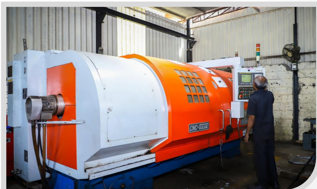
CNC TURNING CENTER TAKANG (MADE IN TAIWAN) D 400 X 2000 L MM
