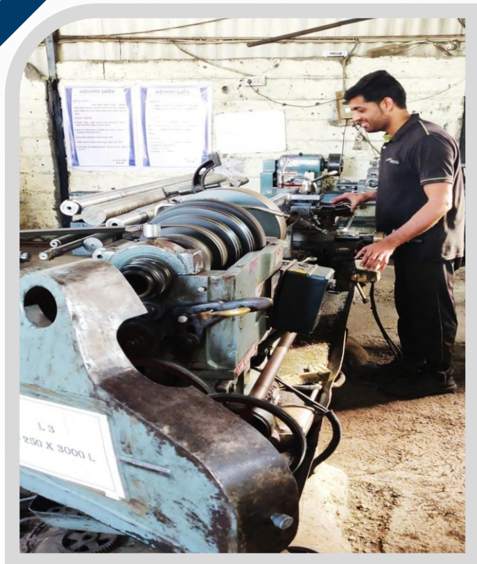
MAX CENTER LATHE (MADE IN RAJKOT ) D 400 X 3700 L MM
