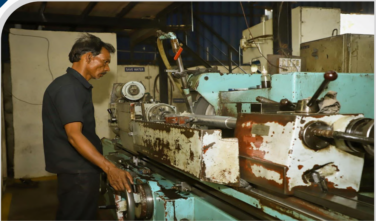
TOSS CYLINDRICAL GRINDING ( MADE IN CZECHOSLOVAKIA ) D 200 X 2000 L MM
