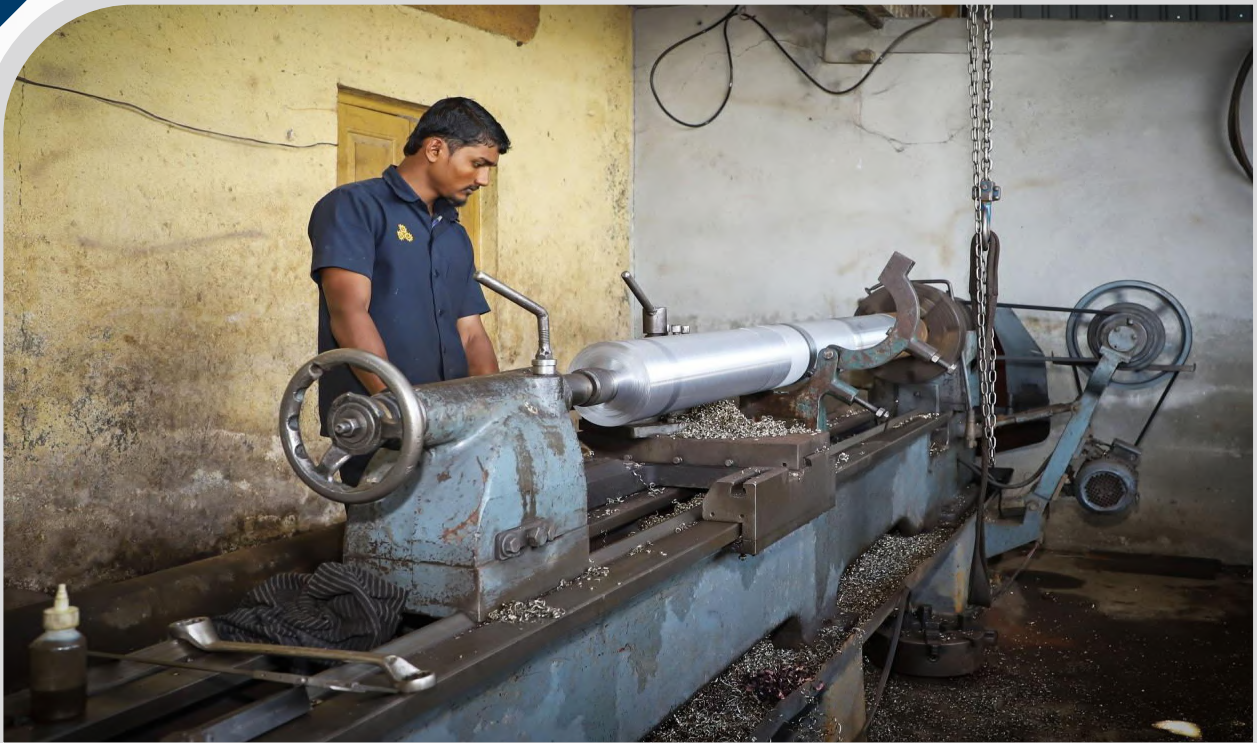
STAR CENTER LATHE MACHINE (MADE IN RAJKOT) D 250 X 4000 MM L
