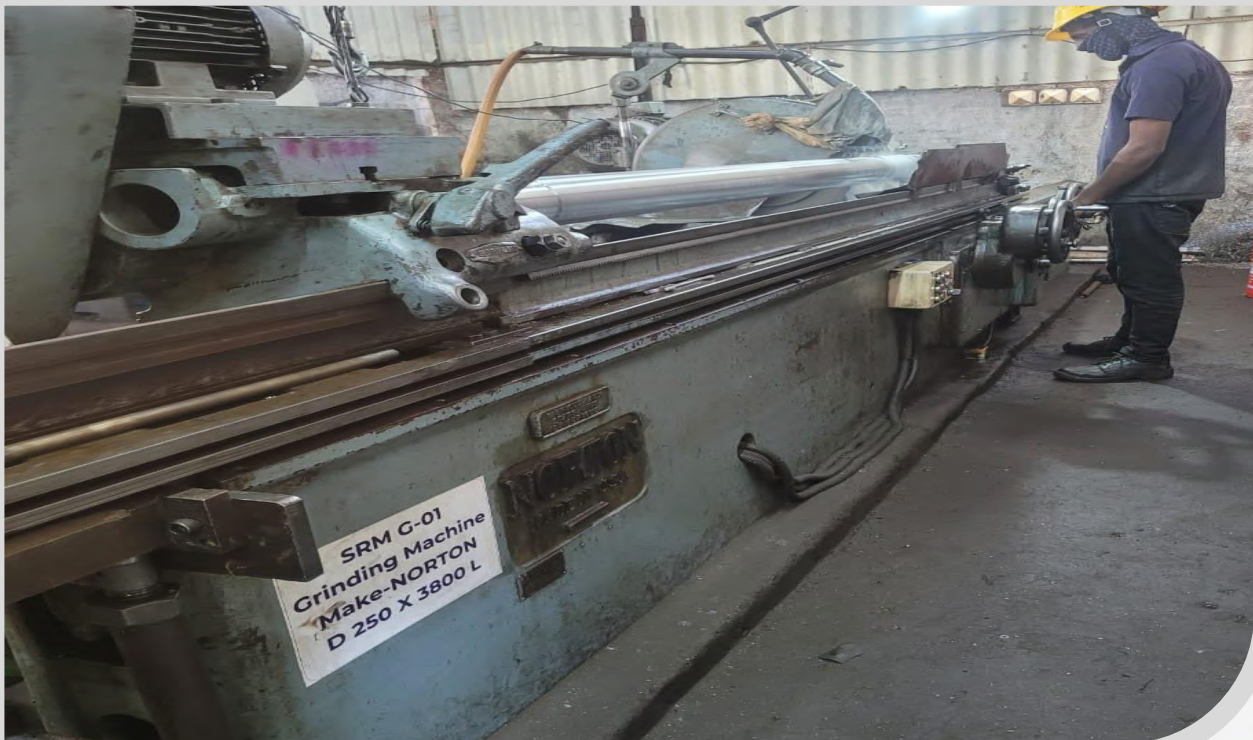
NORTON CYLINDRICAL GRINDING ( MADE IN U.S.A ) D 280 X 3700 L MM
