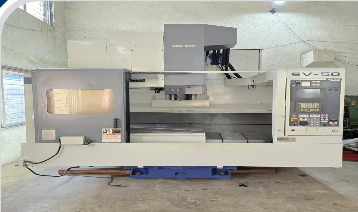
VMC MACHINE. MORI SEIKI (MADE IN JAPAN) ( D500X1300MM)
