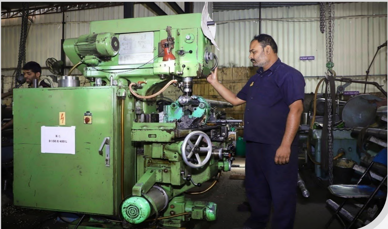
HURTH KEY WAY MILLING ( MADE IN GERMANY ) D 290 X 400 L MM
