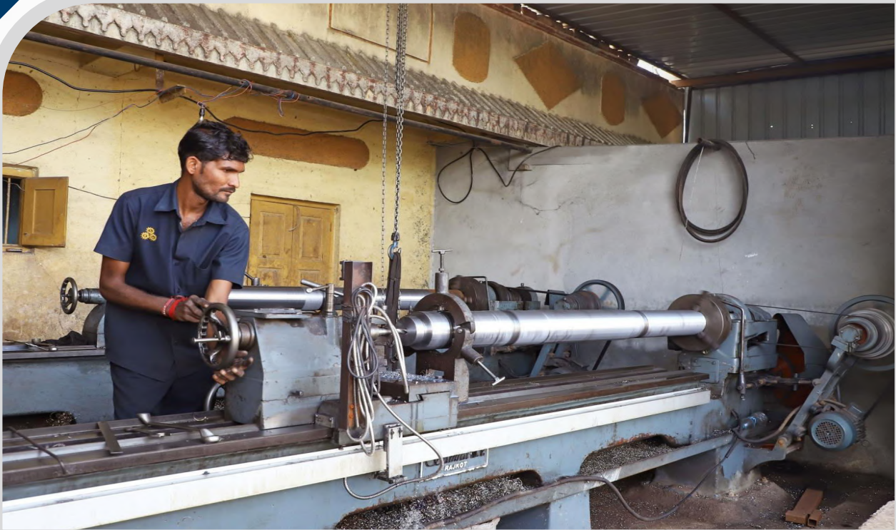
RAVI CENTER LATHE MACHINE ( MADE IN RAJKOT ) D 250 X 4000 MM L
